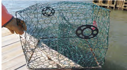
Figure 93: Biodegradable Panels in Crab Traps
