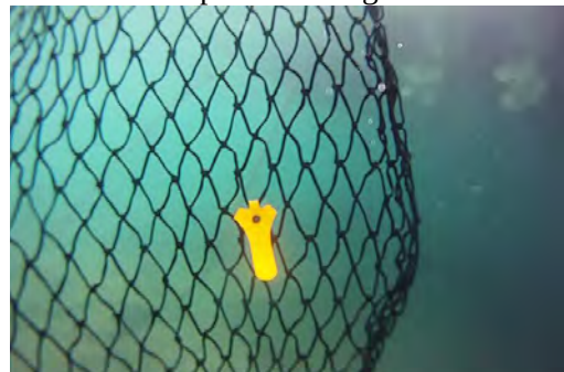
Figure 92: Biodegradable Purse Seine with Radio Chip
