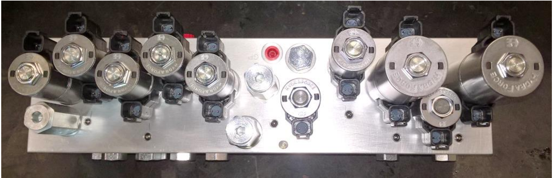
Boom manifold showing the solenoid coils and valves
