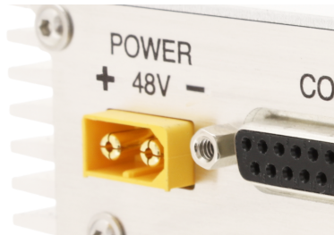
Drawing of the connector from the laser side.
