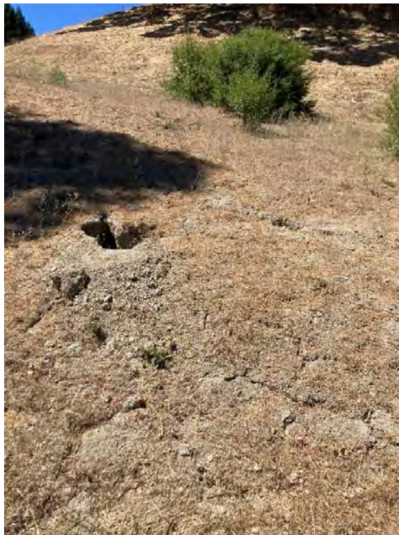
Photo 14. View of an animal burrow within shallow slope failure.
