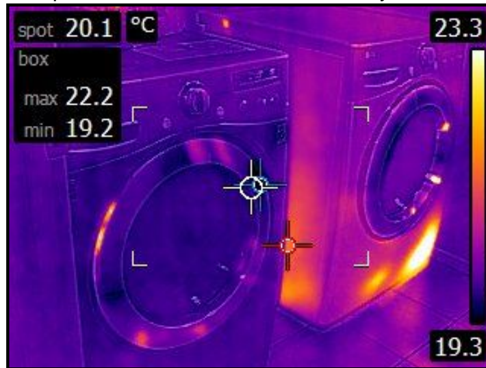
Appliances scanned for leaks - no issues to report
