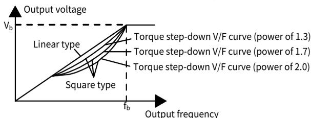
**Note:** In the figure,  $V_b$  indicates the motor rated voltage and  $f_b$  indicates the motor rated frequency.
