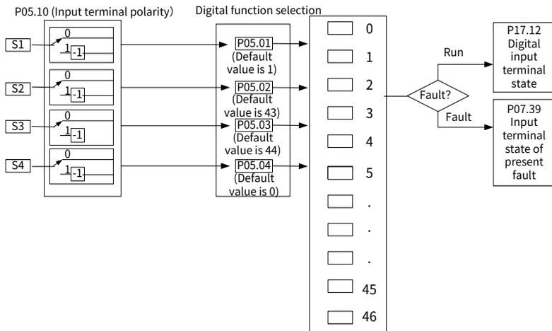
**Note:** Two different multifunction input terminals cannot be configured with a same function.
