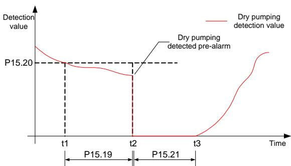
In case of the dry pumping pre-alarm, after the time specified in P15.21, the pre-alarm will be automatically cleared and the machine will restart.
