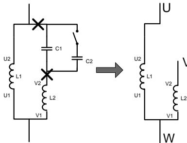
Two-phase control wiring shall strictly align with UVW, and common methods for determining main and auxiliary windings are as follows:
