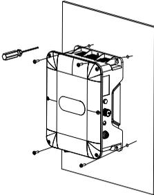
Step 4 Tighten the screws on the wall or mounting plate.
