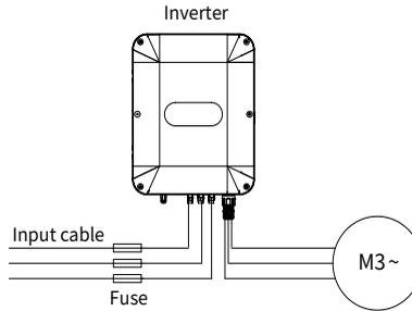
**Note:** Select the fuse according to section [D.2 Breaker and electromagnetic contactor](#).
