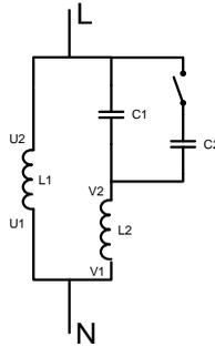
The internal wiring diagram of single-phase motor winding is as follows after removing the starting capacitor and operating capacitor:
