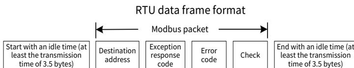
The following table describes the standard structure of an RTU frame.
