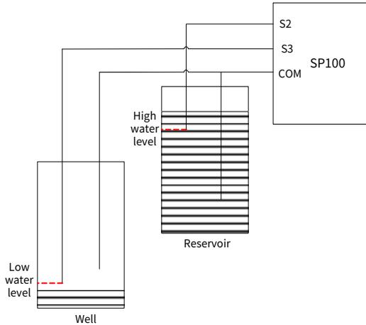
In case of the empty-water pre-alarm, if the water level drops below the high water level warning line, the pre-alarm will be cleared automatically after P15.15, and the machine will restart.
