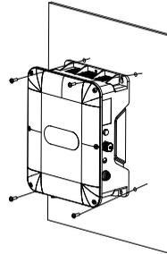
Step 3 Fix the inverter on the wall or mounting plate.
