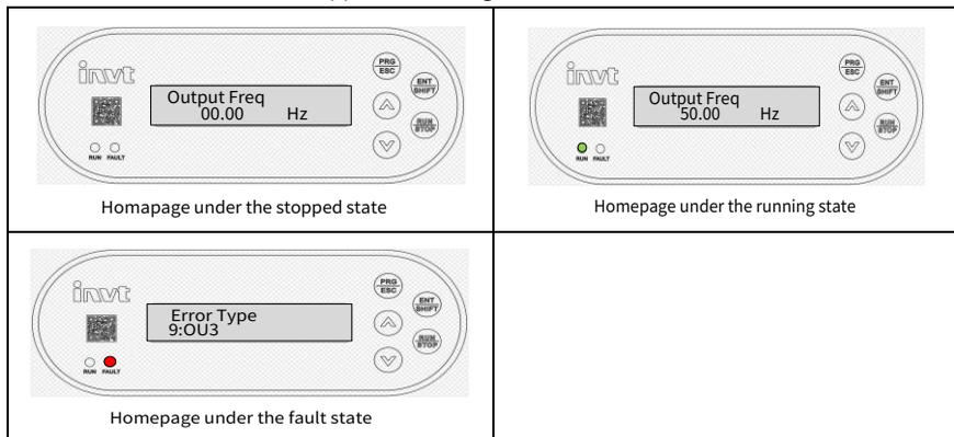
When a fault is detected, the keypad displays the fault code and the fault indicator is on. You can perform fault reset by using the
