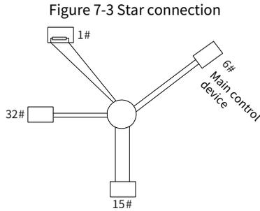
Use shielded cables, if possible, in multi-device connection. The baud rates, data bit check settings, and other basic parameters of all the devices on the RS485 line must be set consistently, and addresses cannot be duplicated.
