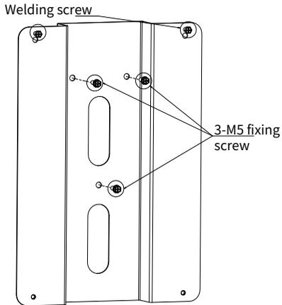
Step 2 Attach the machine (welding screw) to the security plate with screws on the plate.
