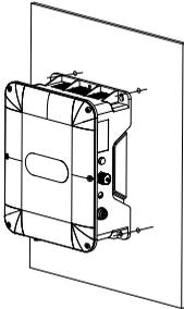
Step 2 Mount the screws or bolts onto the designated positions.
