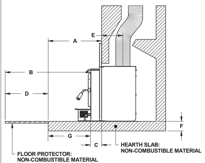
Figure 12: Additional Floor Protection - Not Raised Installation
