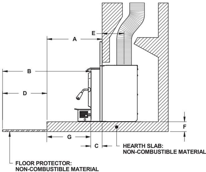
Figure 14: Additional Floor Protection - Raised Installation
