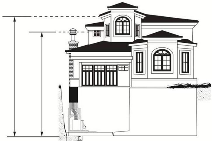
Outside chimneys will lead to cold back drafting when there is no fire in the insert, slow kindling of new fires, and smoke roll-out when the door is open for loading.
