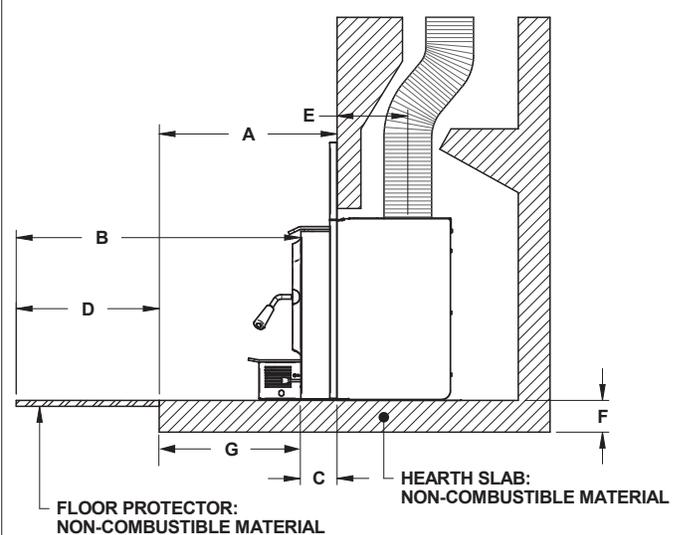
Figure 15: Additional Floor Protection - Not Raised Installation
