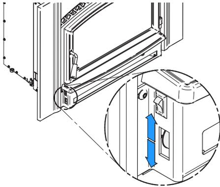
The blower has a variable speed rheostat that can be adjusted from high (HI) to low (LO) and closed (OFF).
