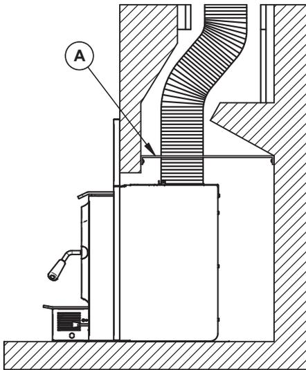
Figure 16: Block-off Plate
