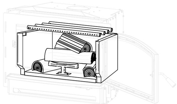
The images above show the space in the firebox where the logs are to be placed. It is important to always respect this space and not to put logs in the grid area marked with an X. The marked area is defined by the space between the glass and the cast-iron andiron. To have a good ignition, place the two lower logs in a north-south position and cross the others on top. Leave enough space between the logs for good air circulation. The log length recommended for this fireplace is 16 in.
