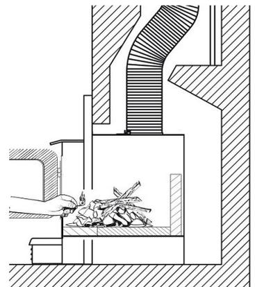
*Do not leave the insert unattended when the door is slightly open. Always close and latch the door after the fire ignites.*
