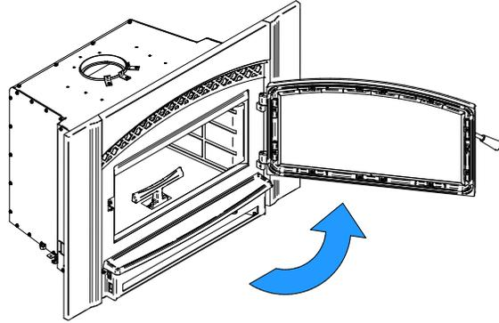
2. Hold the fire screen by the two handles and bring it close to the door opening.
