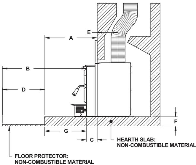
Figure 11: Additional Floor Protection - Raised Installation
