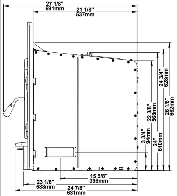
Figure 2: Side View - Minimum Insert Projection
