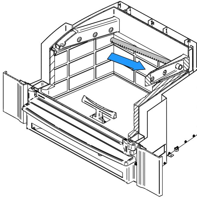
2. Align the notch in the left end of the tube with the key of the left air channel hole. Using a «Wise grip» hold the tube and lock it in place by turning the tube as shown. Make sure the notch reaches the end of the key way. Repeat for center back tube.
