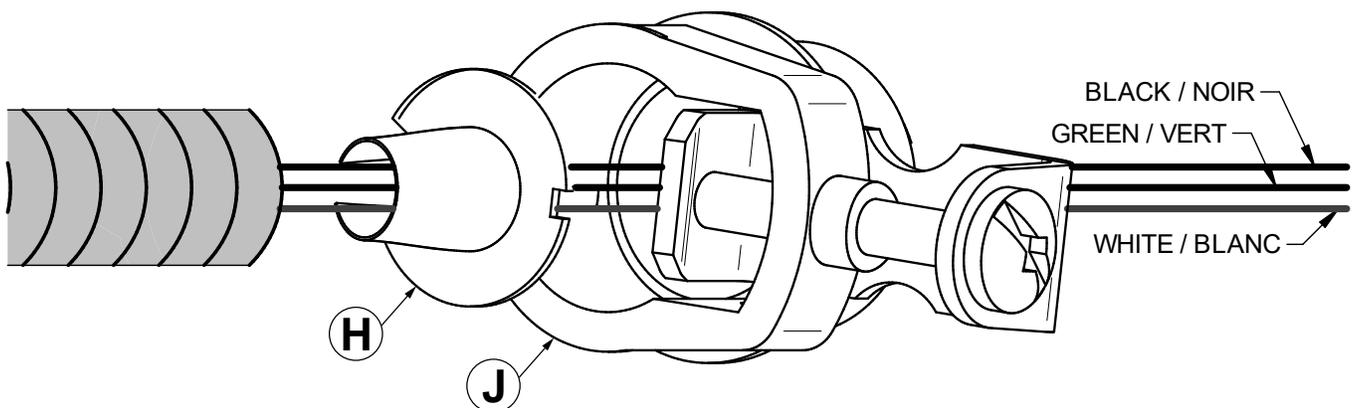
8. Install the connector (**J**) on the insert.
