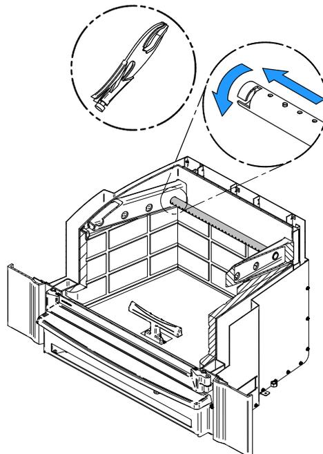
Note that secondary air tubes (A) can be replaced without removing the baffle board (B). See exploded view for tube installation order.
