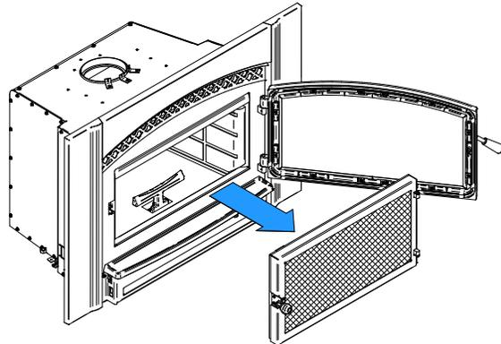
3. Lean the upper part of the fire screen against the top door opening making sure to insert the top fire screen brackets behind the primary air deflector.
