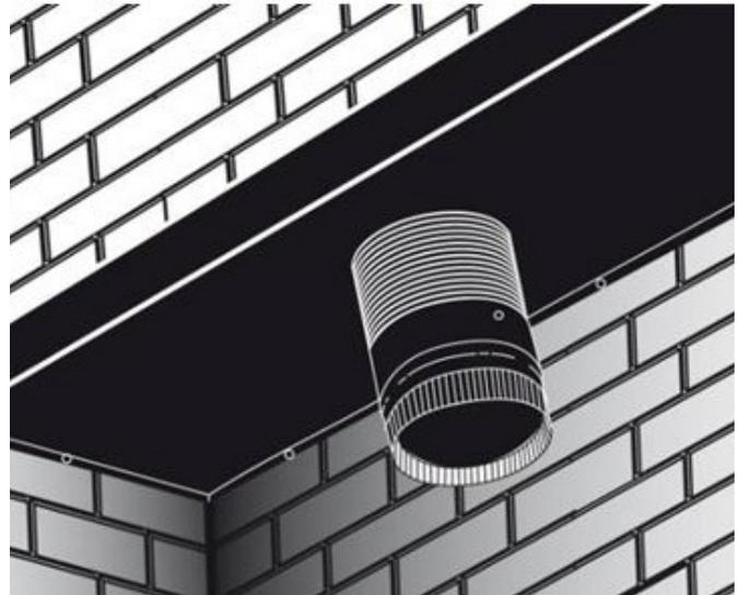
Figure 17: Block-off Plate
