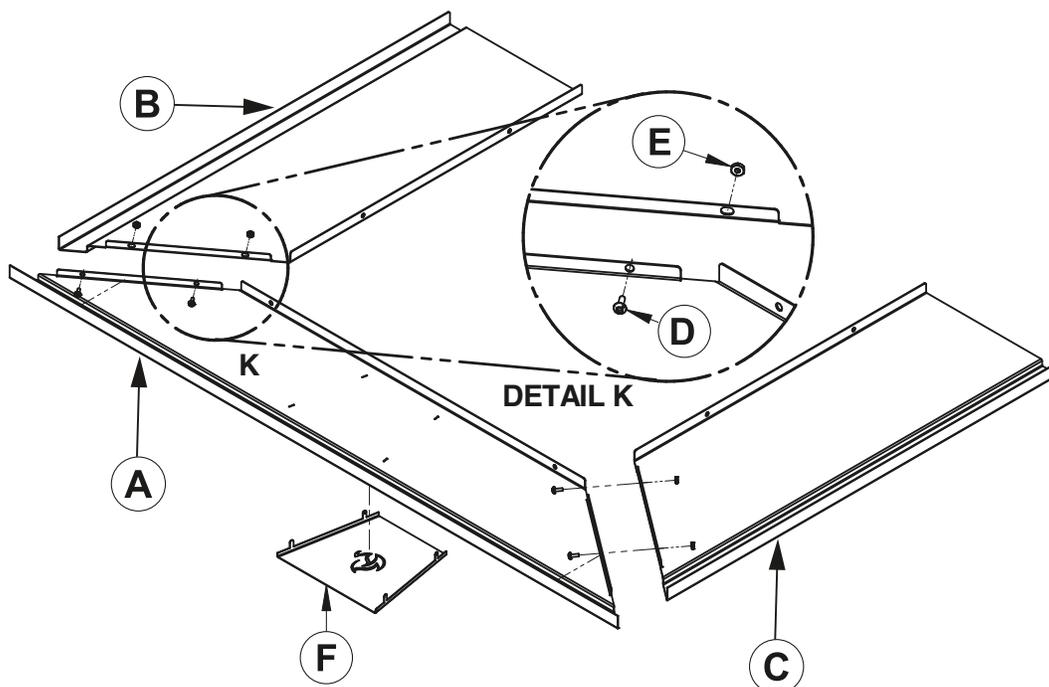
2. Place the faceplate panels with the finished side down on a flat, soft, non-abrasive surface. Line up the holes of the upper faceplate panel (**A**) with the holes of the side panels (**B**) and (**C**). Secure them together using four bolts (**D**) and nuts (**E**) provided. Insert the plate (**F**) in the slots at the center of the upper faceplate panel (**A**).
