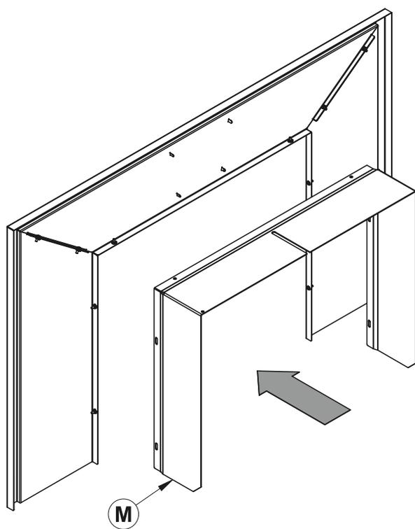
7. Align the holes in the faceplate extension **(M)** with the holes in each faceplate side panels.
