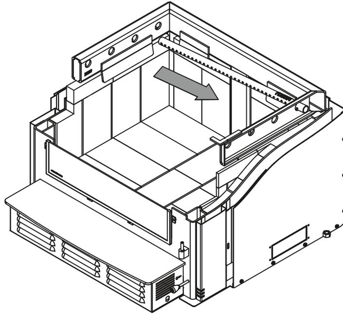
2. Align the notch in the left end of the tube with the key of the left air channel hole. Using a « Wise grip » hold the tube and lock it in place by turning the tube as shown. Make sure the notch reaches the end of the key way.
