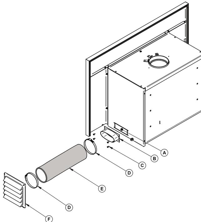
2. Install the fresh air intake adapter **(B)** with four screws **(C)** then secure the flexible pipe<sup>19</sup> **(E)** (not included) to the adapter **(B)** using one of the pipe clamps **(D)**. Secure the other end of the pipe to the outside wall termination **(F)** using the other pipe clamp **(D)**. The outside wall termination **(F)** must be installed outside of the home.
