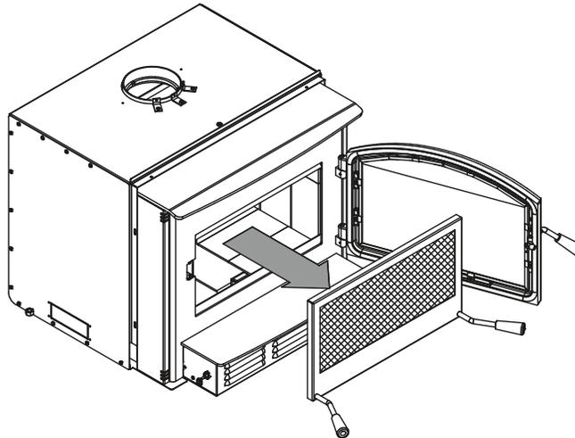
3. Lean the upper part of the fire screen against the top door opening making sure to insert the top fire screen brackets behind the primary air deflector.
