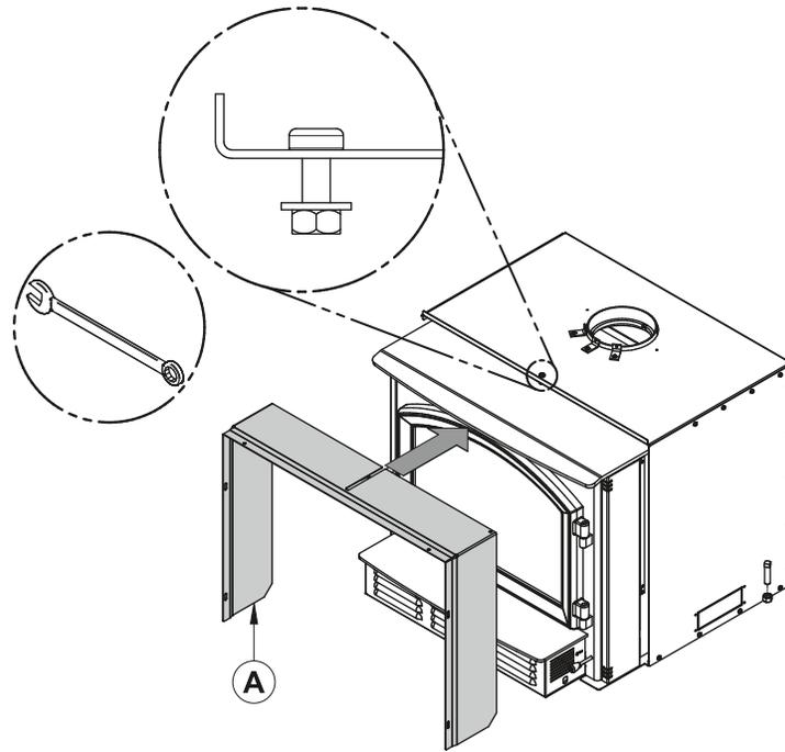
1. Remove the faceplate extension (**K**) secured between the firebox and the convection air jacket.
