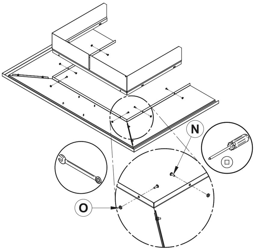
8. Secure both assemblies together using 6 bolts **(N)** and nuts **(O)** provided.
