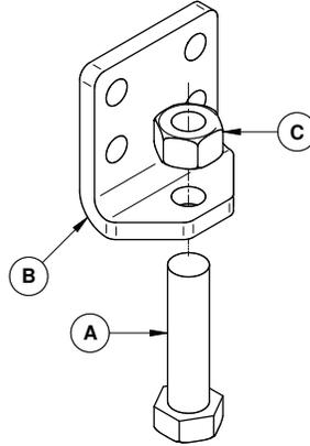
2. Install the leveling system on both side at the back of the unit with 2 screws (D) using a power drill with a 5/16» hex head.
