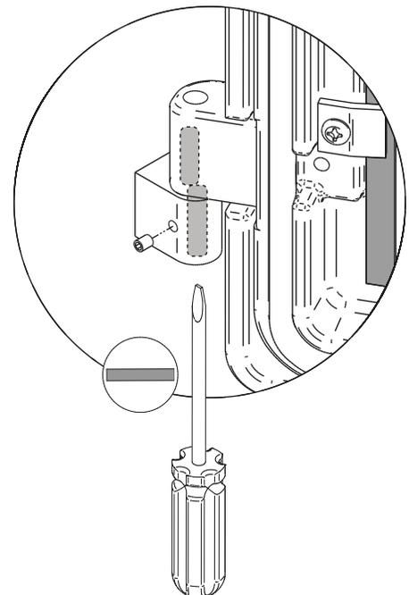
Using a flat screwdriver, turn the adjustable hinge rods in the direction shown to adjust the doors. Tighten all door hinge pressure screws when they are at the desired positions. Configurations 1-2-3-4-5-6, show in which direction these act on the adjustment of the door.
