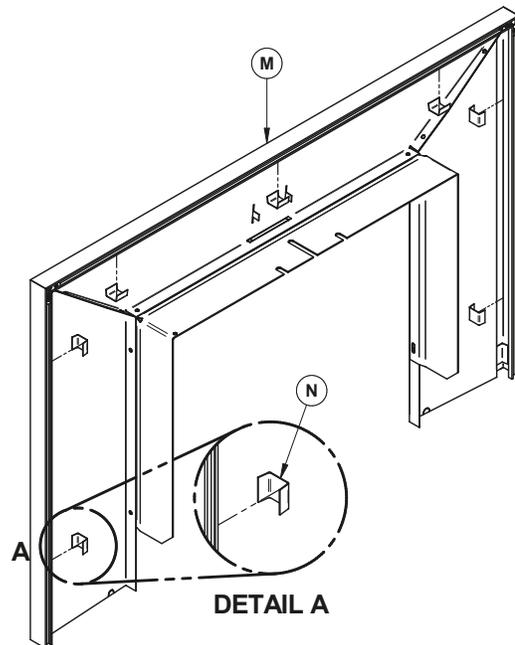
5. Align the trim assembly with the left and right edge of the faceplate and slowly slide it down over the faceplate.
