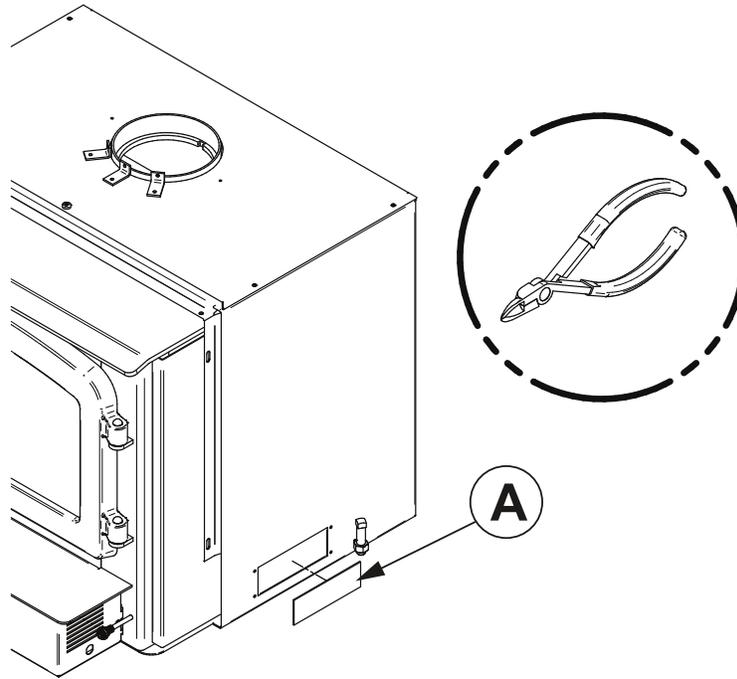
1. Using pliers, remove the rectangular metal plate **(A)** retained by the micro-seals to clear the opening for the outside air intake.
