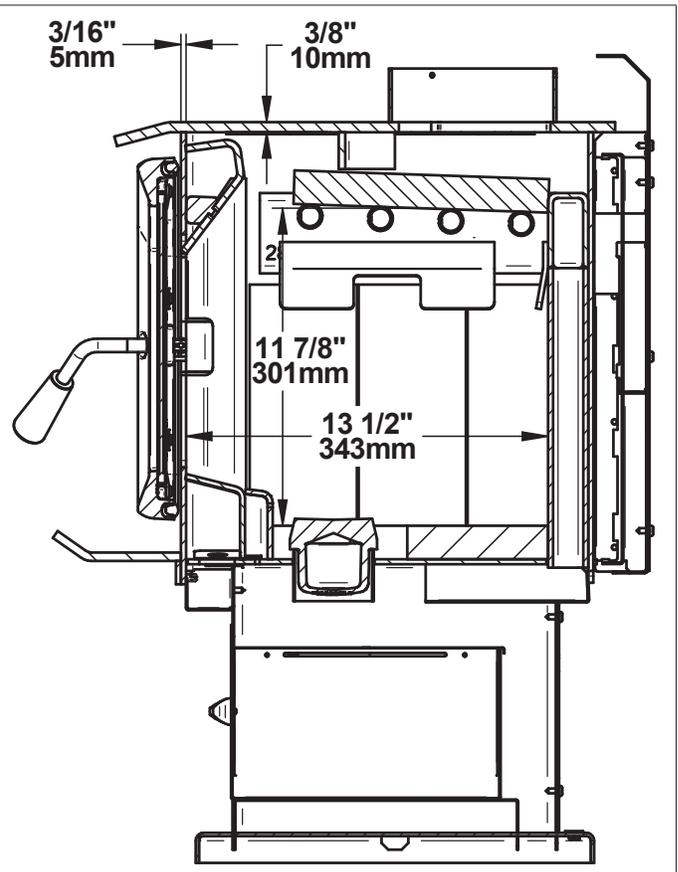
Figure 15: Side View - Combustion Chamber
