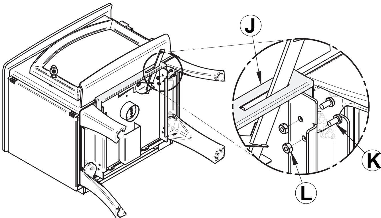
6. Put the stove on its legs, install the ash drawer included with the kit. Put back the firebricks, the ash plug and the door on the stove. See step 1.
