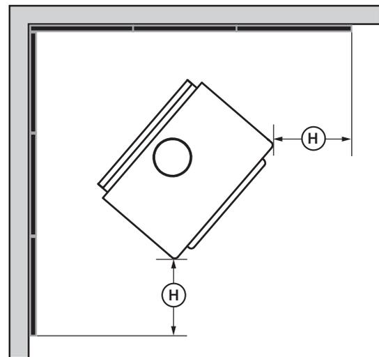
Figure 35: Heat shield clearances
