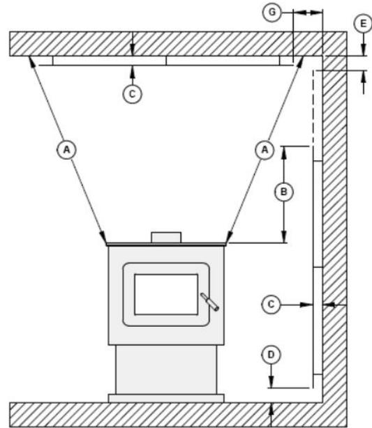
Figure 33: Heat shield clearances
