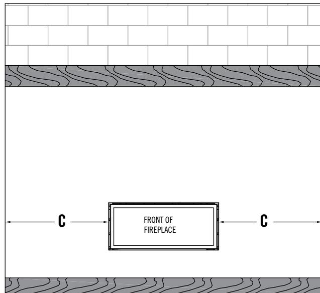
The width of the overhang to each side of the appliance (C) must be a minimum of 1/2 or greater of the roofline elevation (B) above the base of the fireplace.
