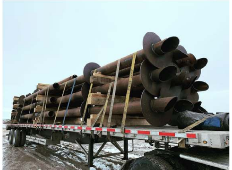
A tractor trailer transported these high-capacity helical piles. Smaller piles can be hauled by a heavy-duty
