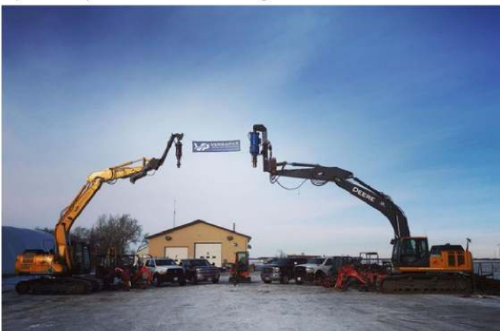
A "family photo" of some of the equipment we use to install helical piles at VersaPile.
