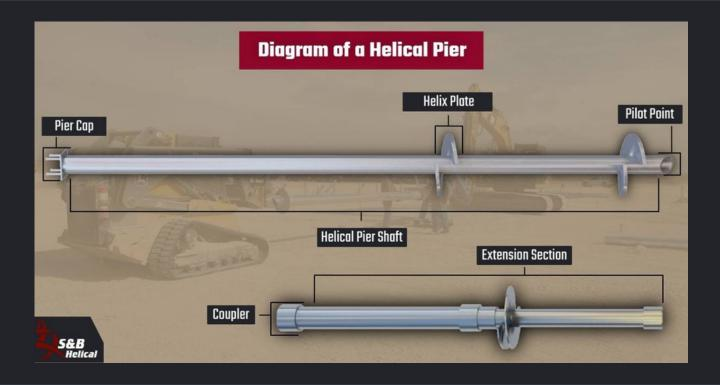
As the pier is installed by being turned into the ground, the soil begins to exert pressure on the helix plates (and the pier shaft, to a lesser extent).
