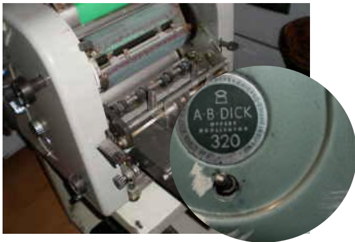
The A.B. Dick Tabletop Offset Model 320 first introduced in 1959
