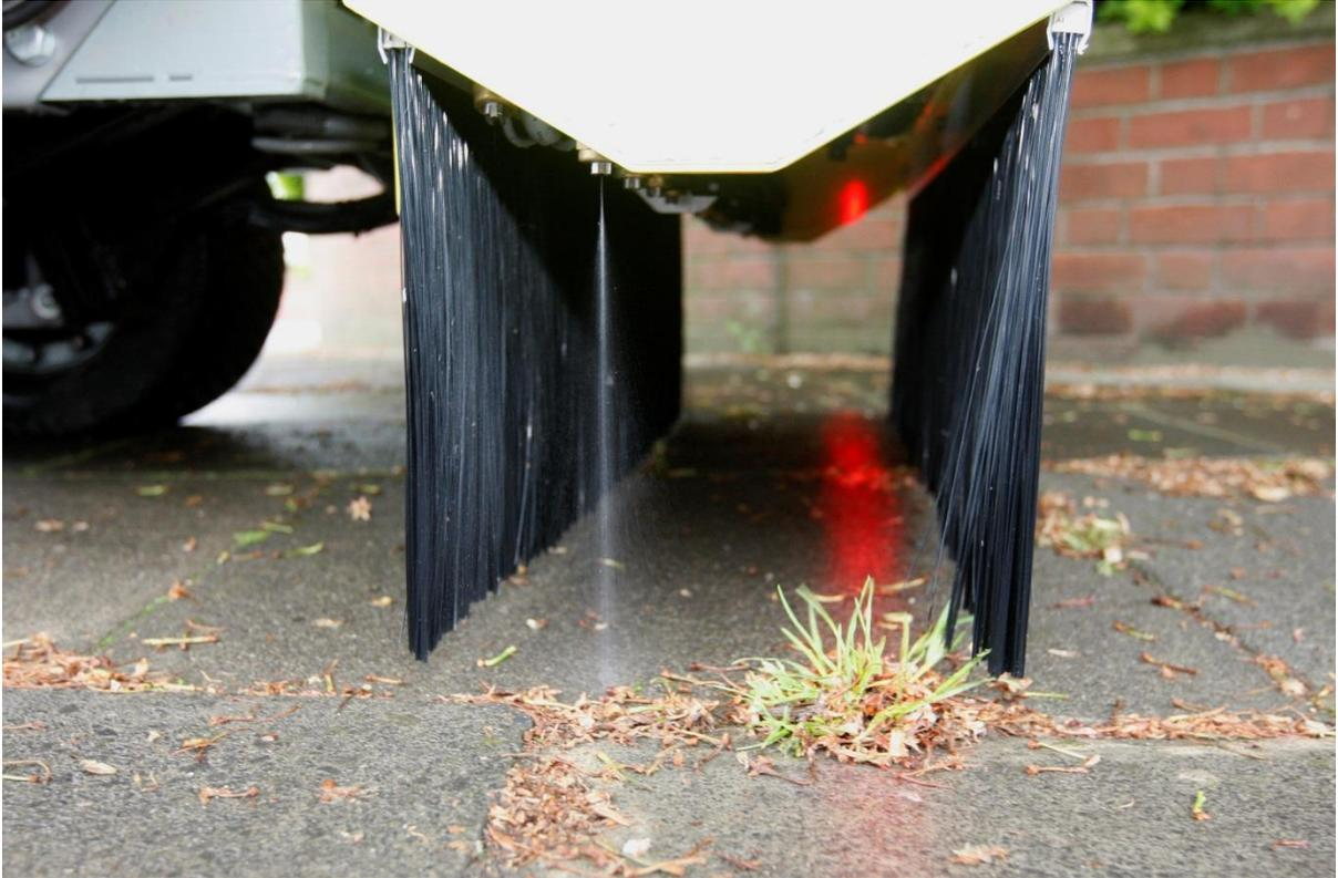
The machine was compared with a hand operated sprinkle bar and a knapsack sprayer. Tests were carried out on three types of hard surface and two levels of weed infestation.
